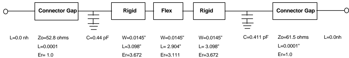
Figure 6. Equivalent Circuit for Rigid-Flex Test Coupon
